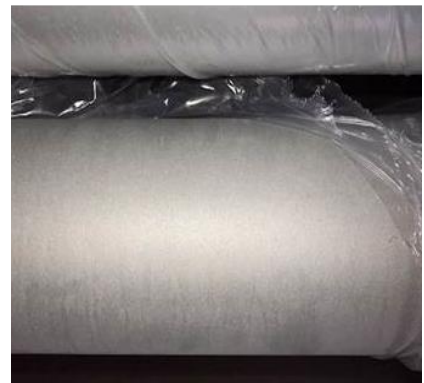
Figure C: Uniform surface of pipe visible after grit blasting.
